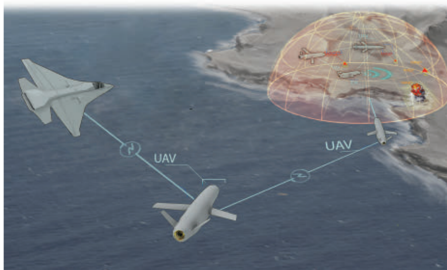
Pictured is an artist’s concept of the CODE program’s focus on improving collaborative autonomy, or the capability of groups of unmanned aircraft systems (UAS) to work together under one person’s supervisory control.
