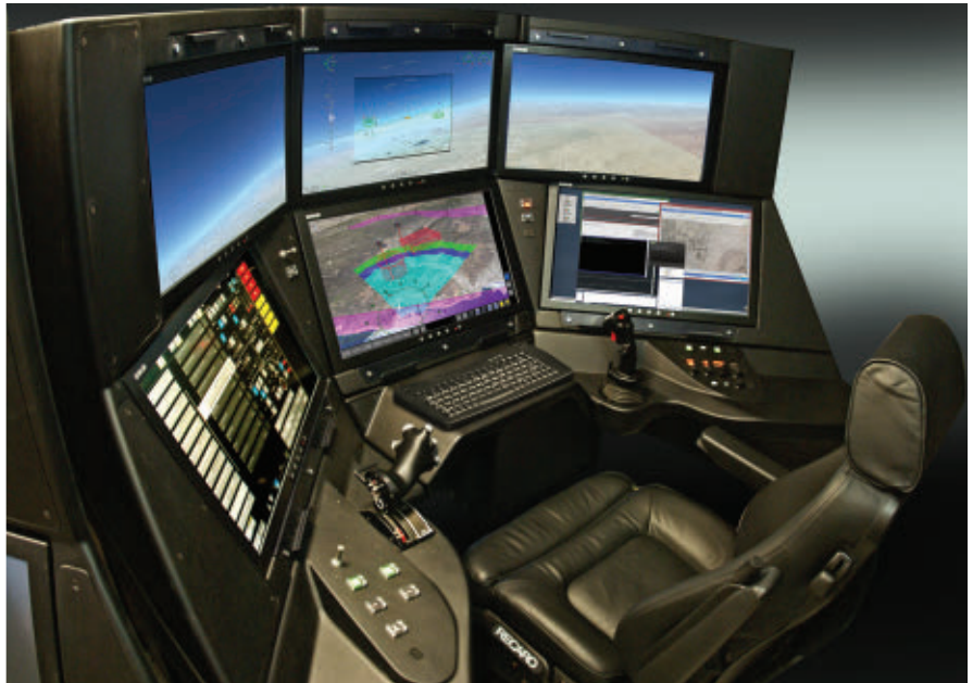
As part of its initiative to certify a remotely piloted aircraft to fly in national airspace, General Atomics is creating a certifiable ground control station for MQ-9B pilots.
